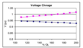
Fig. No. 7 Change in voltage in bus no. 6 with increased reactive load
