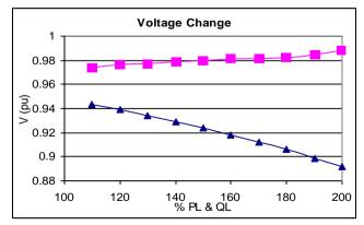
Fig. No. 8 Change in voltage in bus no. 6 with increased system load
