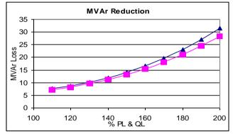
Fig. No. 6 Reactive power loss with increase in system load
